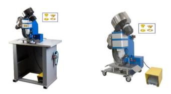
Automatic, pneumatic eyelet machine for Metal eyelets and washers. Places eyelets and washers on all types of materials: textile, cardboard, canvas, PVC, etc. It has two independent feeders and boxes with big capacity. For eyelets and metal washers up to 13 mm inner diameter. Pierce the material and rivet the eyelets in the same movement with two independent axes, do not wrench the material. With stainless steel tray with guides to adjust the distance between eyelets.
