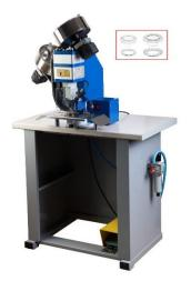
Automatic, pneumatic eyelet machine with double feeding, for plastic eyelets and washers from Jopevi (10 mm, 12 mm, or 16 mm). Places eyelets and washers on all types of materials: textile, cardboard, canvas, PVC, etc. Two independent feeders for eyelets and washers of great capacity. Punches the material and rivet the eyelets in the same movement with two independent axes, do not wrench the material. With stainless steel tray with guides to adjust the distance between eyelets.
