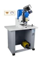
Motor driven automatic eyelet machine with one guide to set eyelets. By changing the rail, you can place metal eyelets between 6 mm and 22 mm inner diameter. It has a feeder for large capacity of eyelets. Punches the material and rivet the eyelets in a single movement with two independent axes, do not wrench the material. With laser pointer to place the eyelets on all types of materials: leather, textile, cardboard, canvas, PVC, etc.
