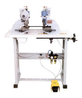
Automatic pneumatic machine with double head to put two rivets in folder rings. Places rivets on all types of materials: footwear, plastic, textile, cardboard, canvas, PVC, etc.
